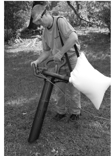
Figure 4-9: Picking up debris with vacuum
